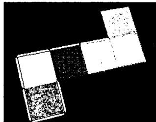
Figure 10. The 2D shape that results from unfolding the cube in a sequence different from that shown in Figure 8. Creation of "flippers" in partially-automated design of packaging, also with flippers added.
